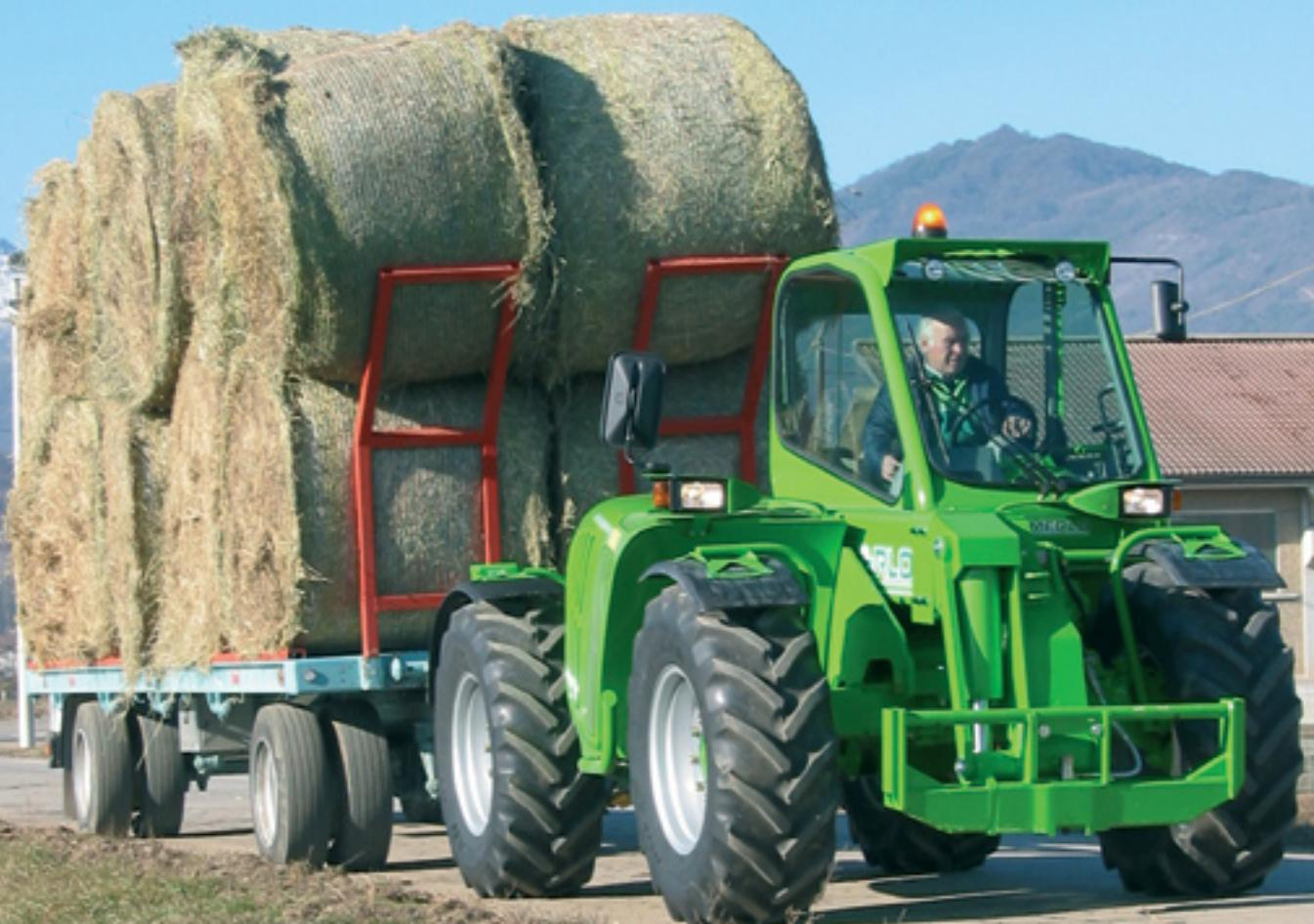
**Homologated in Europe as an agricultural tractor with up to 20 tonnes towing capacity (depending upon local road regulations).**
